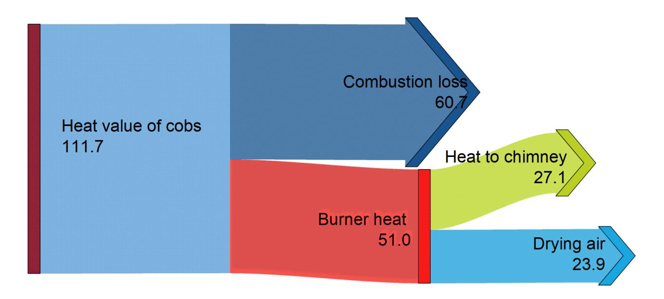
Fig. 2: Heat energy balance for maize cobs drying in MJ (Basis = 1 hour).
