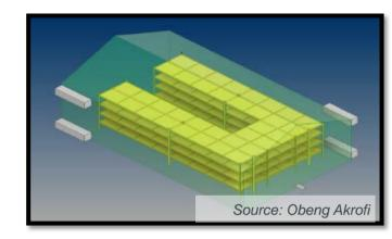
Several drying levels on 4 to 5 shelves for different types of produce to be dried
