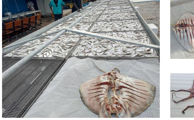
Loading of the Solar tunnel dryer
