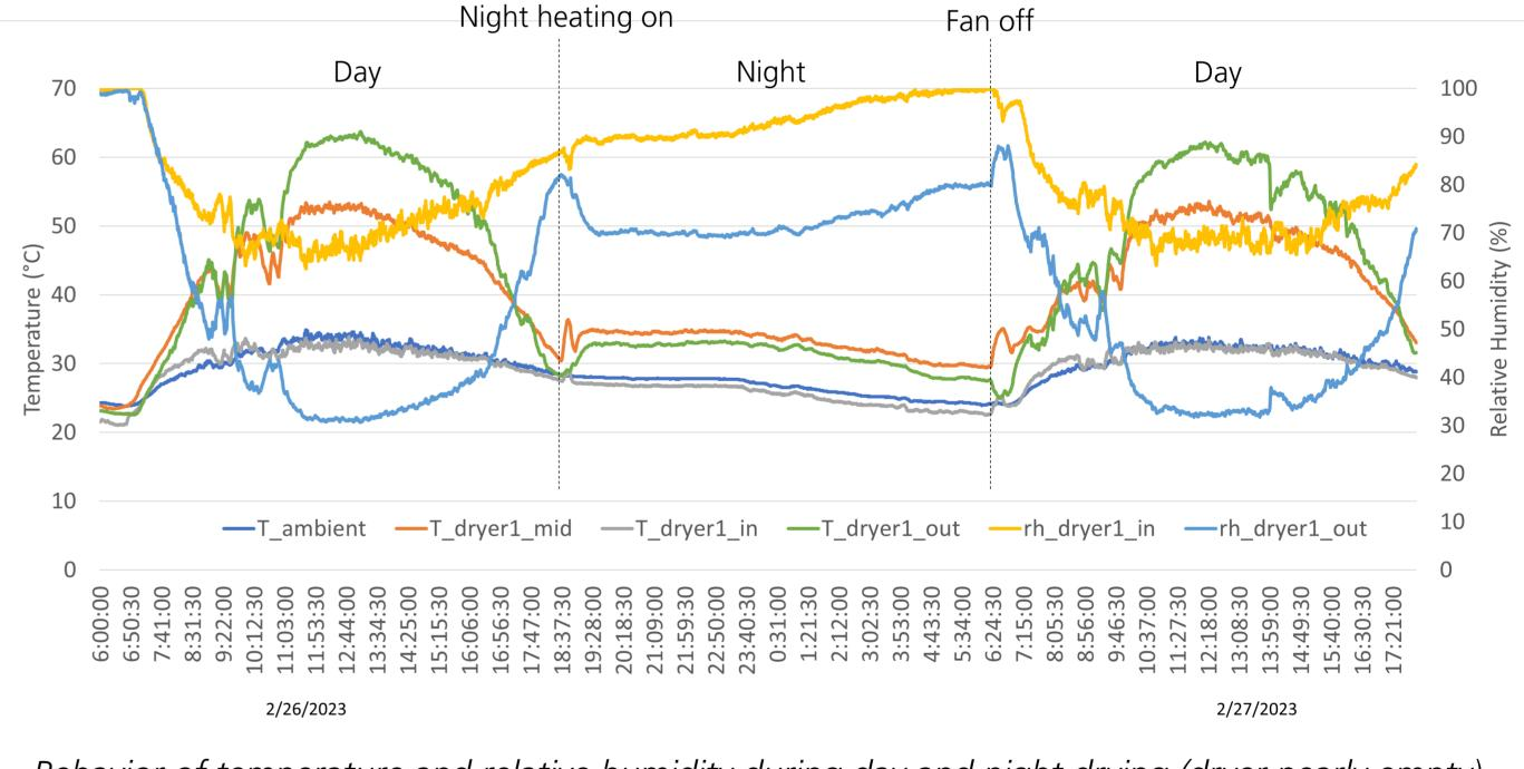
Behavior of temperature and relative humidity during day and night drying (dryer nearly empty)
