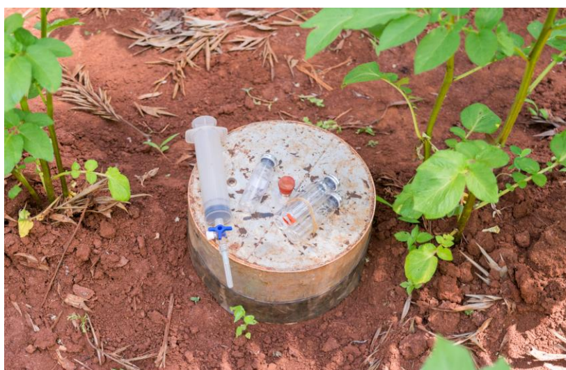
Figure 1: Chamber for greenhouse gas collection
