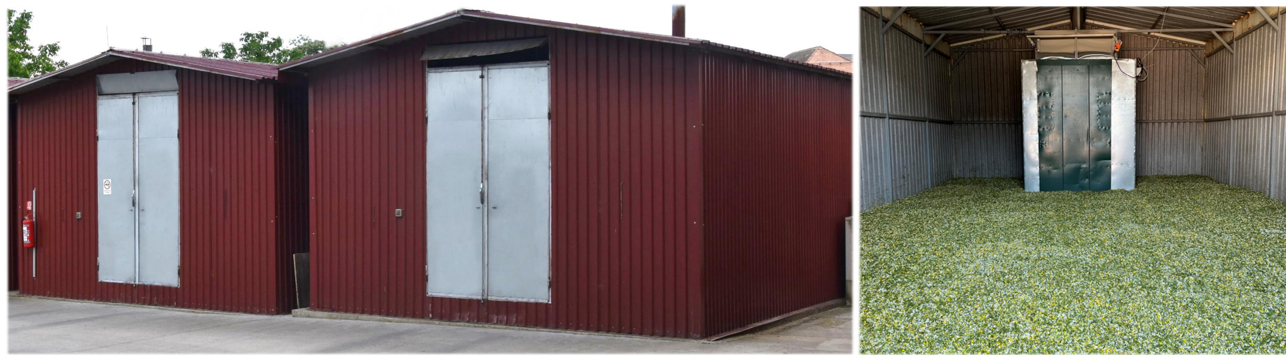
Figure 1. Outside (left) and inside (right) view of the flatbed dryer used for experimental tests
