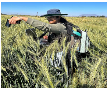
Figure 1: Canopy-level measurements of wheat using an ASD FieldSpec spectroradiometer
