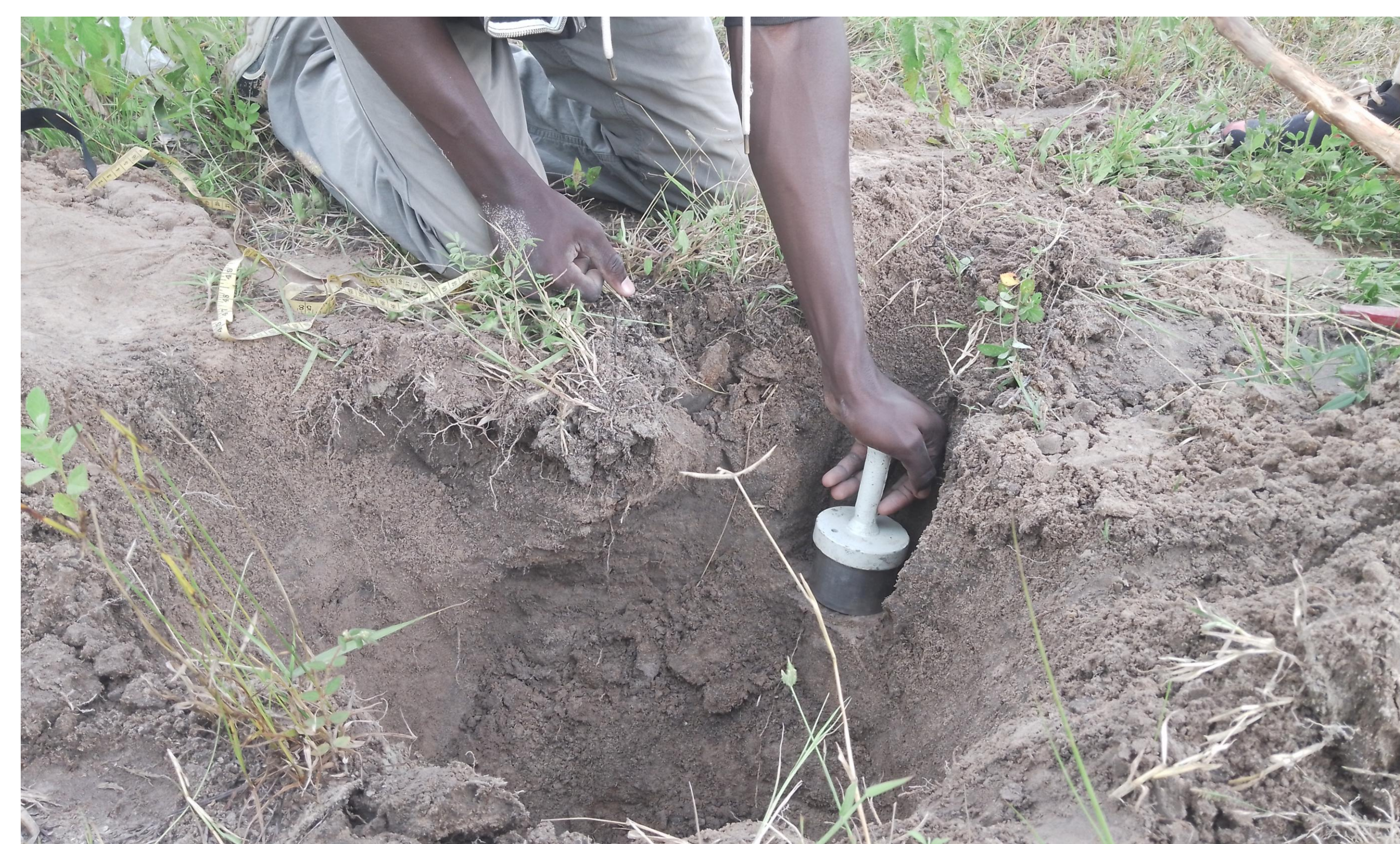
Photo1: Sampling bulk density at the top layer in the head of Mékrou watershed
