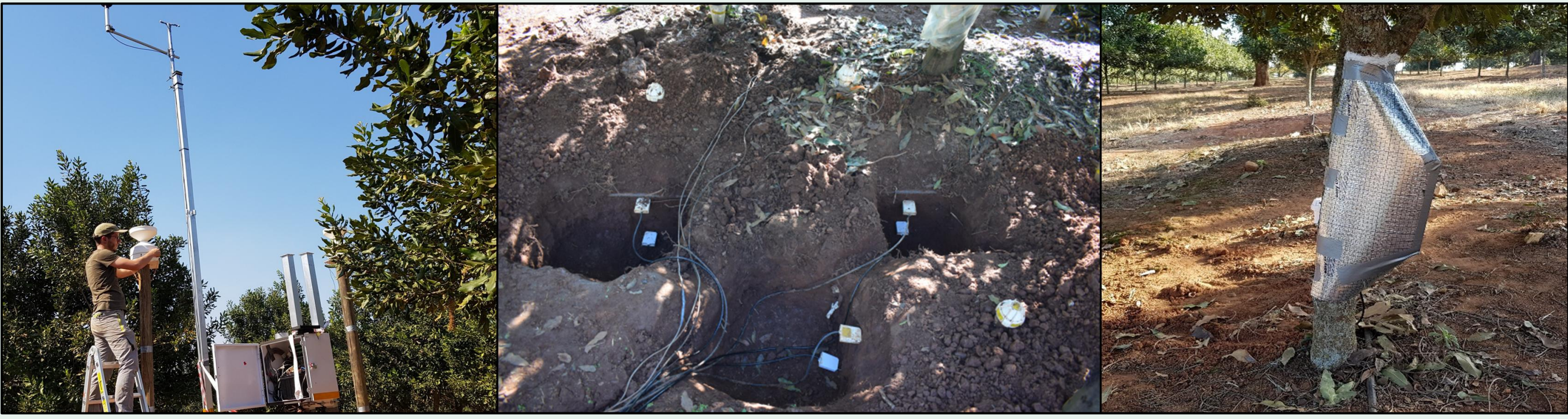
Fig. 2: On-farm measurement of microclimatic parameters, soil water content, and sap flux density. Source: Bringhenti et al. (2025)
