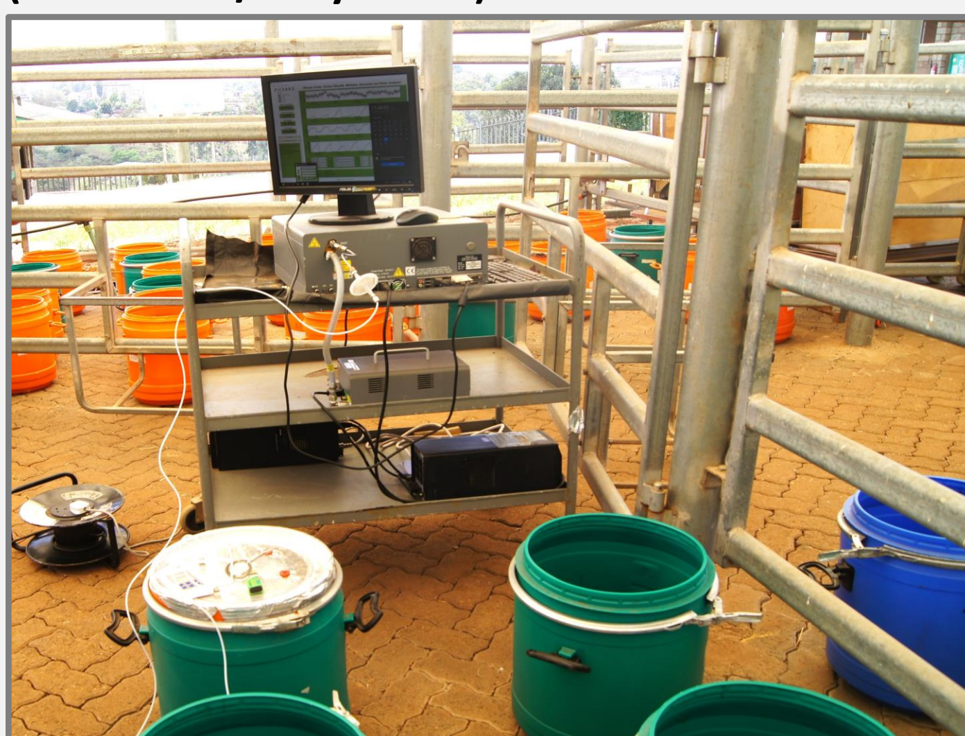
Figure 5: Emissions of ammonia, methane, and nitrous oxide from the manure were measured with a Picarro laser spectrometer. (Photo: ILRI/Chebet Arusey)
