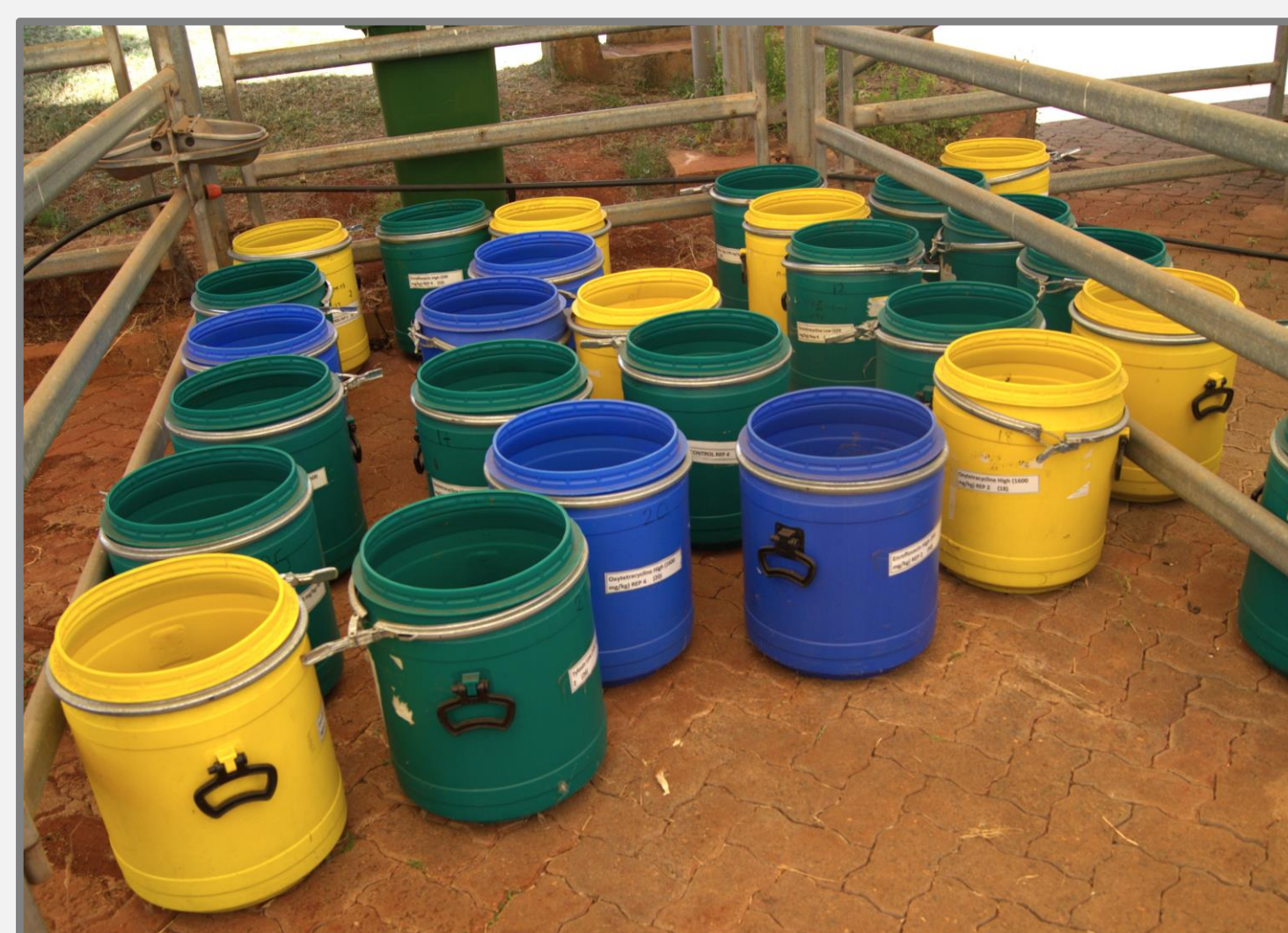
Figure 4: Aliquots of 10 kg fresh cattle manure were incubated in 40 L buckets under a roof outside Mazingira for 105 days. Lids were kept open to allow for ventilation. (Photo: ILRI/Chebet Arusey)
