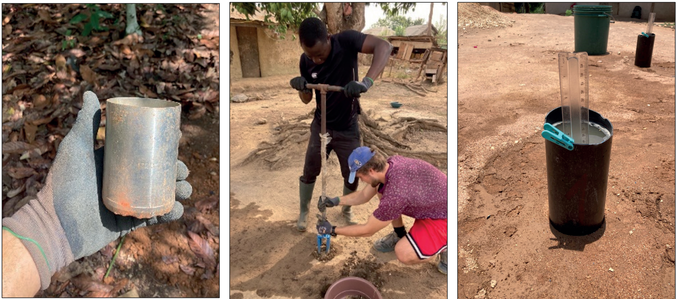
Figure 5: From left to right: Soil sampling of bulk density, texture and infiltration (Kfs)
