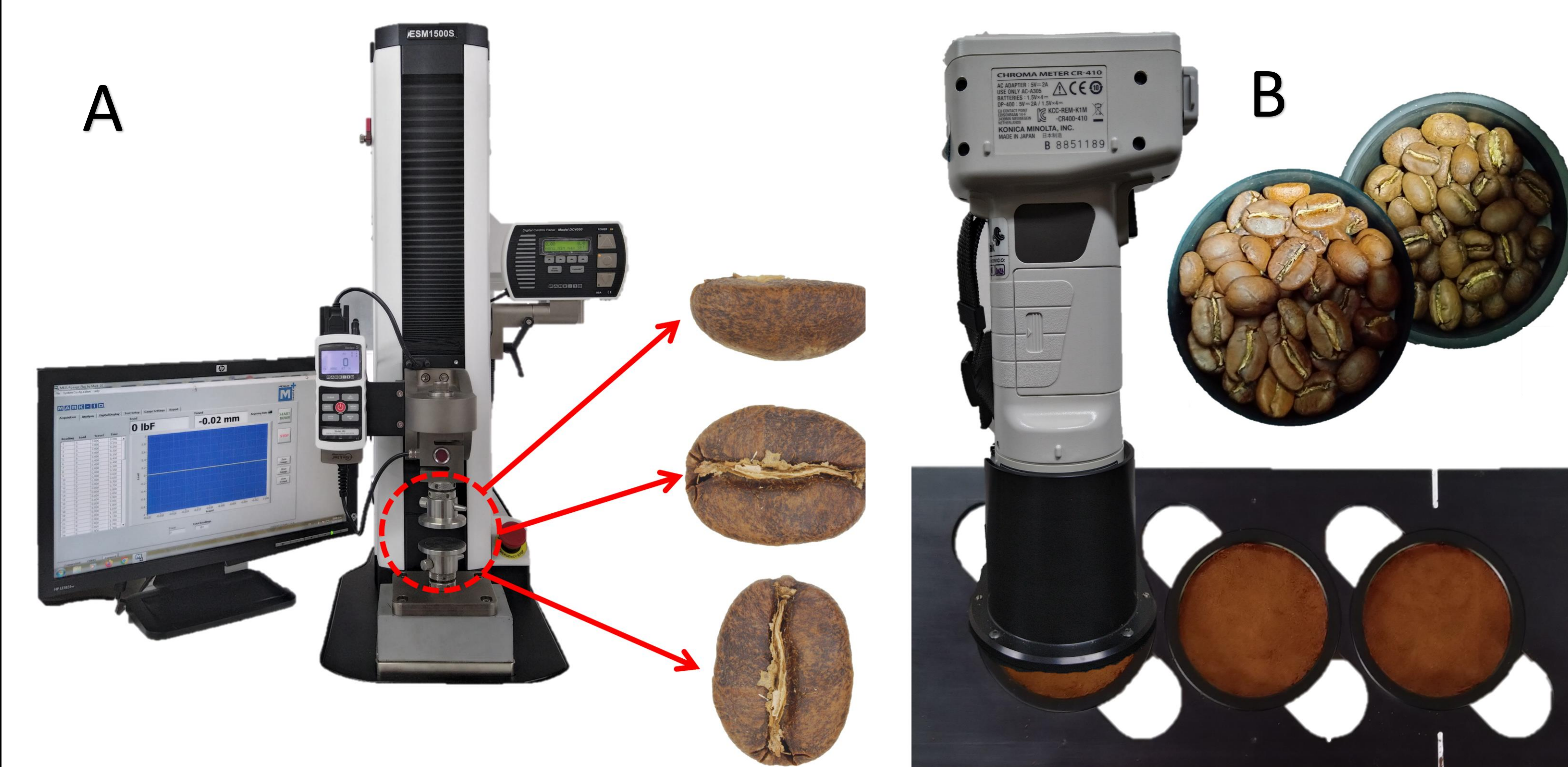
Figure 2. A. Compressive and shear tests. B. Colorimetry
