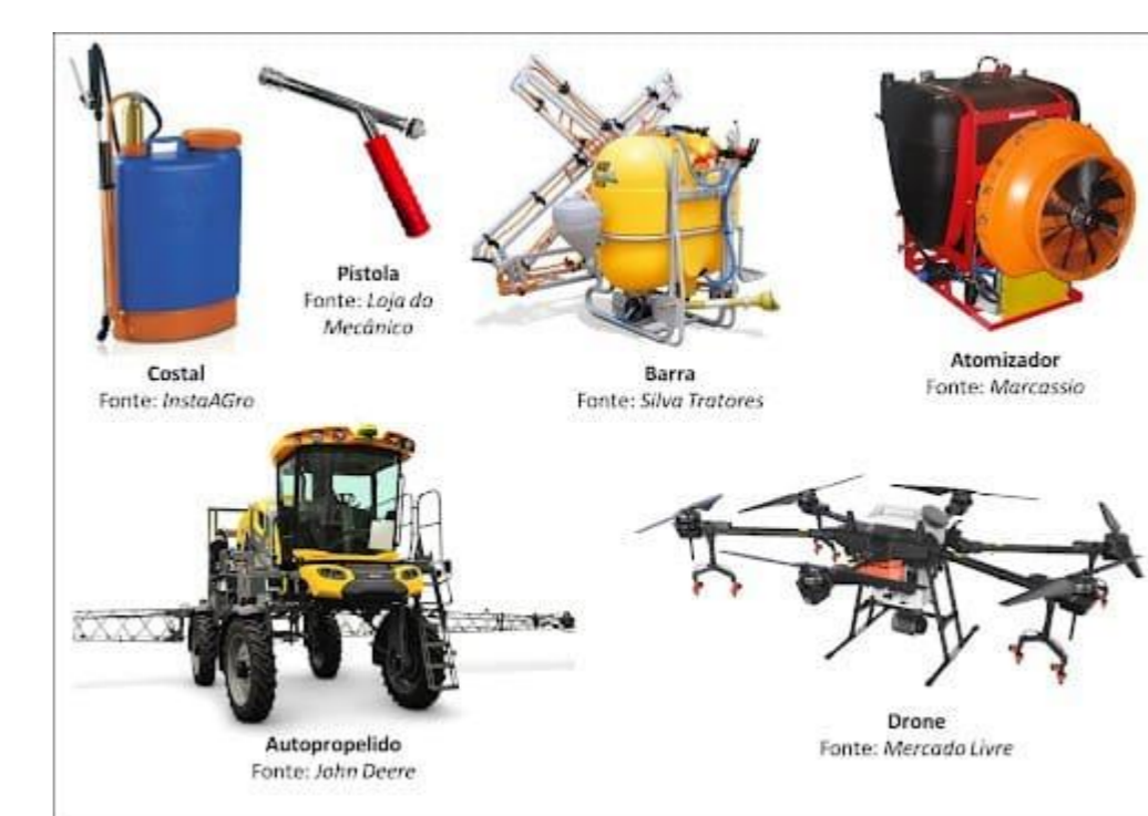
Figure 2: Spraying equipment that could be used to apply the bioinsecticide Lalguard Java in common bean crop.
