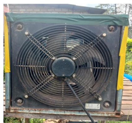
Fan with control system of air speed (1.1 and 2.6 m.s)
