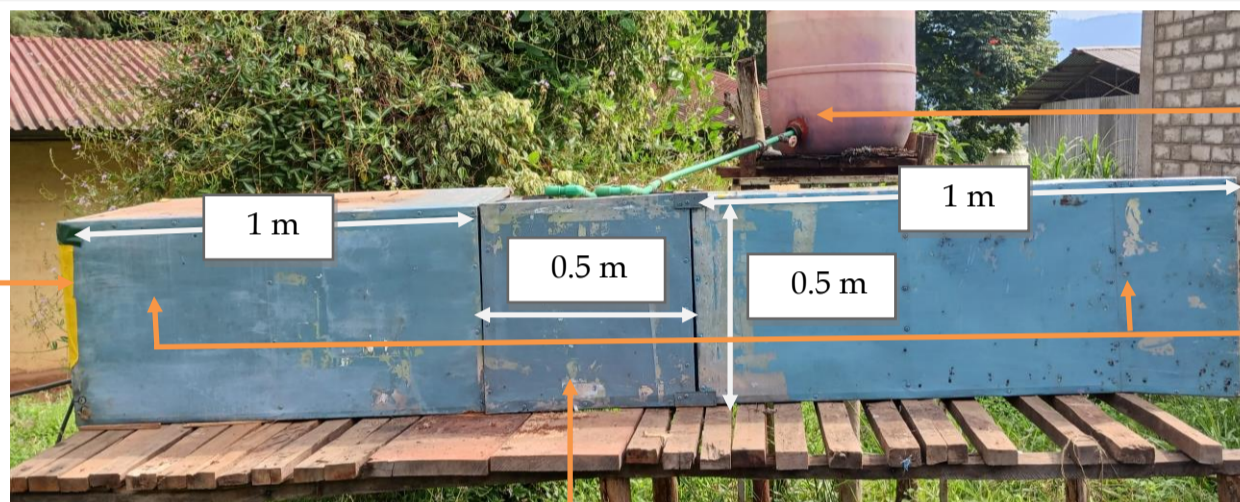
Wet pad made from galvanized sheet, + square steel + Cellulose pad made from False Banana fiber at different thickness (12 - 32 cm) and fiber orientation (Vertical vs Horizontal)
