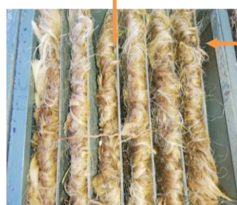
Wet pad made from galvanized sheet, + square steel + Cellulose pad made from False Banana fiber at different thickness (12 - 32 cm) and fiber orientation (Vertical vs Horizontal)
