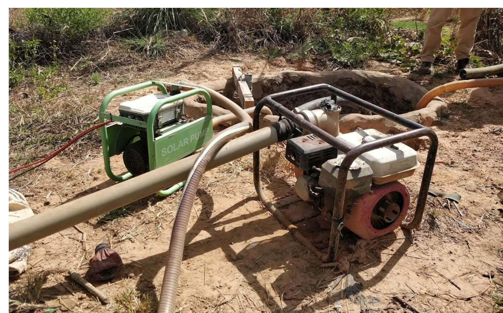
Solar and fuel driven pumps. Photo: J. Schuler
