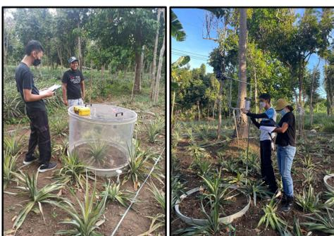
Figure 2. (a) CO<sub>2</sub> and (b) NDVI measurements in the field using developed low-cost DIY devices
