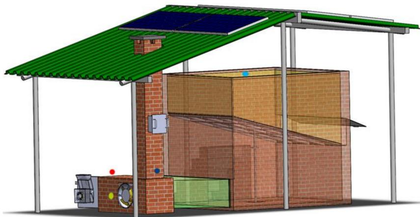
Fig. 1: Technical drawing of the dryer with coloured dots the location of different temperature and humidity sensors
