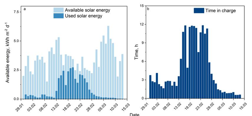
Fig. 4: Solar system performance data records. (a) Yield of the solar system compared to the daily available energy, (b) Total time of charging batteries
