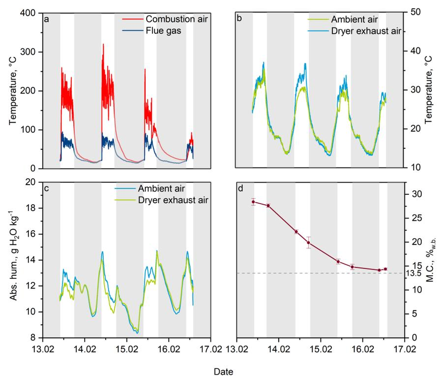
Fig. 3: Temperature of combustion air at outlet of the burner and flue gas in the chimney (a), temperature of the drying air compared to ambient air (b), and the respective absolute humidity (c) shown with drying curves (d)
