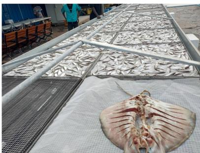
Loading of the Solar tunnel dryer
