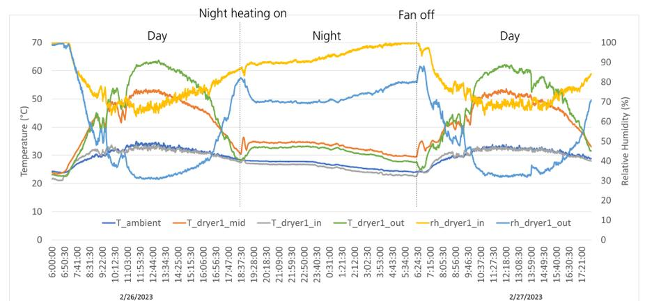
Behavior of temperature and relative humidity during day and night drying (dryer nearly empty)
