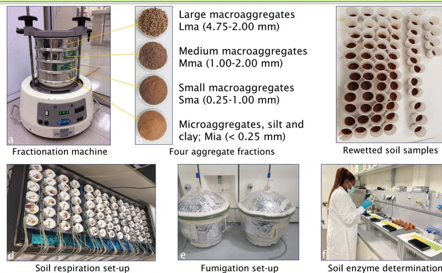
Fig. 3: Physical (a, b) and biochemical (c, d, e, f) laboratory determinations of amended soils
