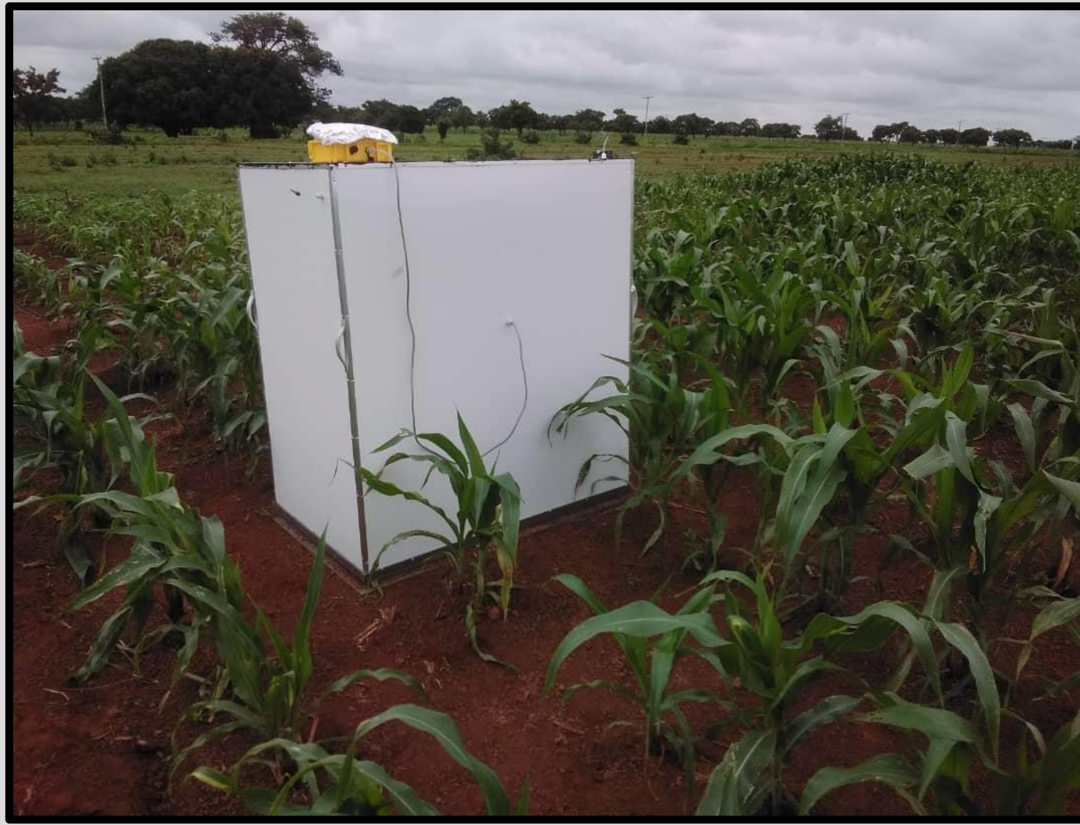
Opaque chamber (measures ecosystem respiration)
