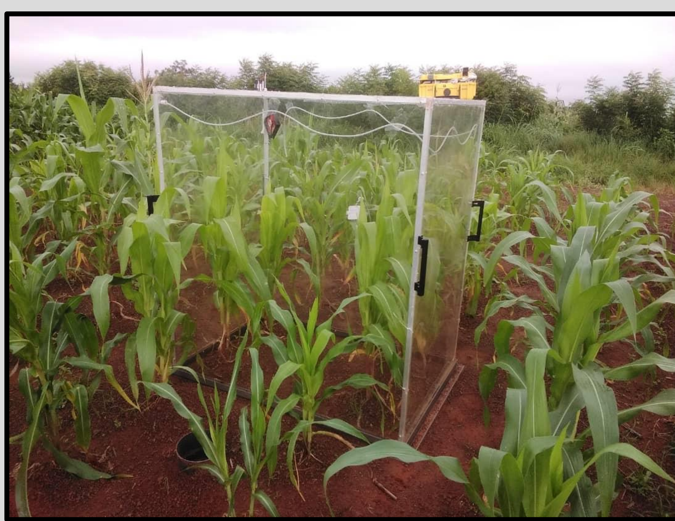
Transparent chamber (measures net ecosystem exchange)
