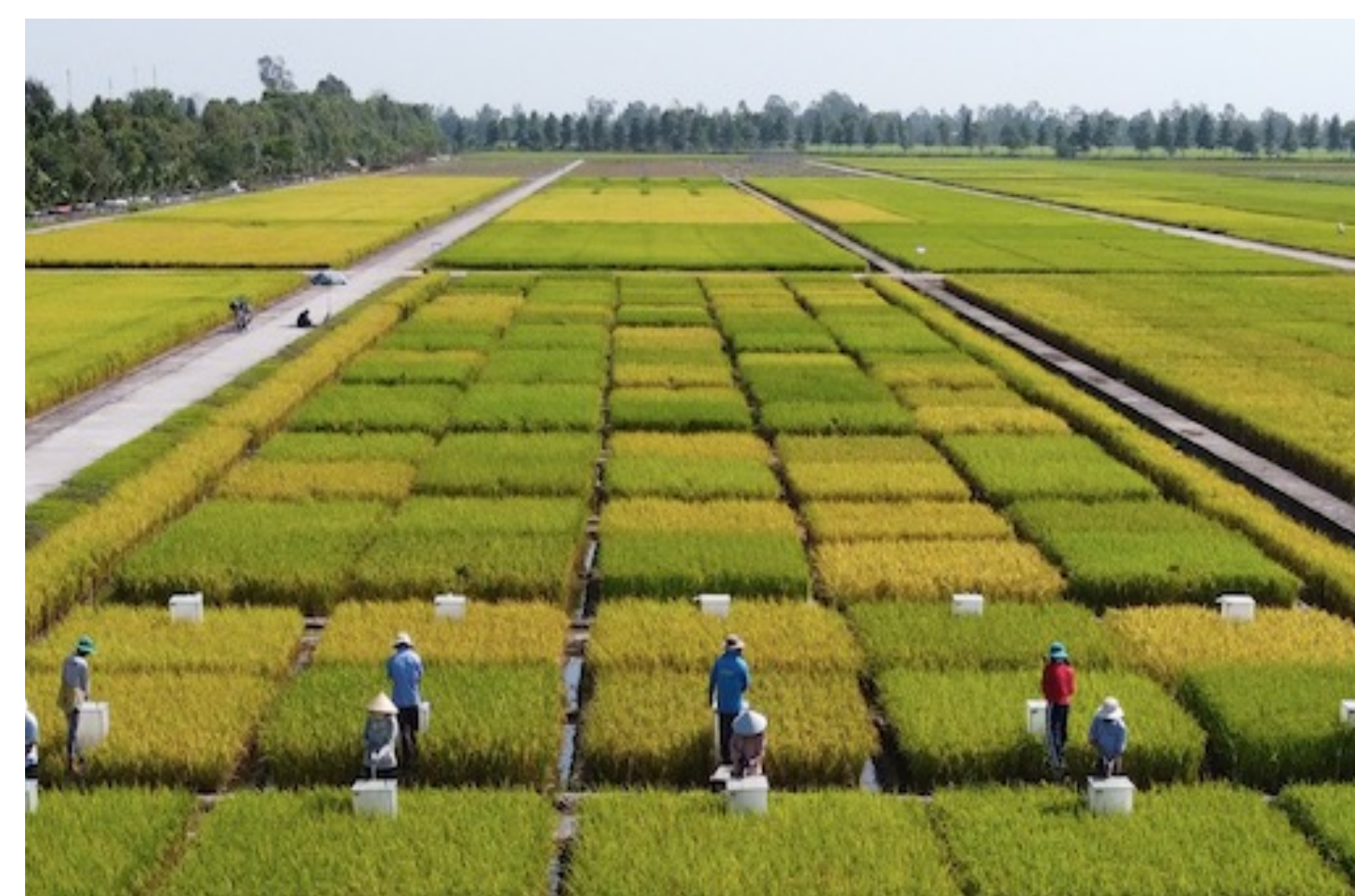
GHG field sampling using the closed chamber method in the Vietnam Mekong Delta
