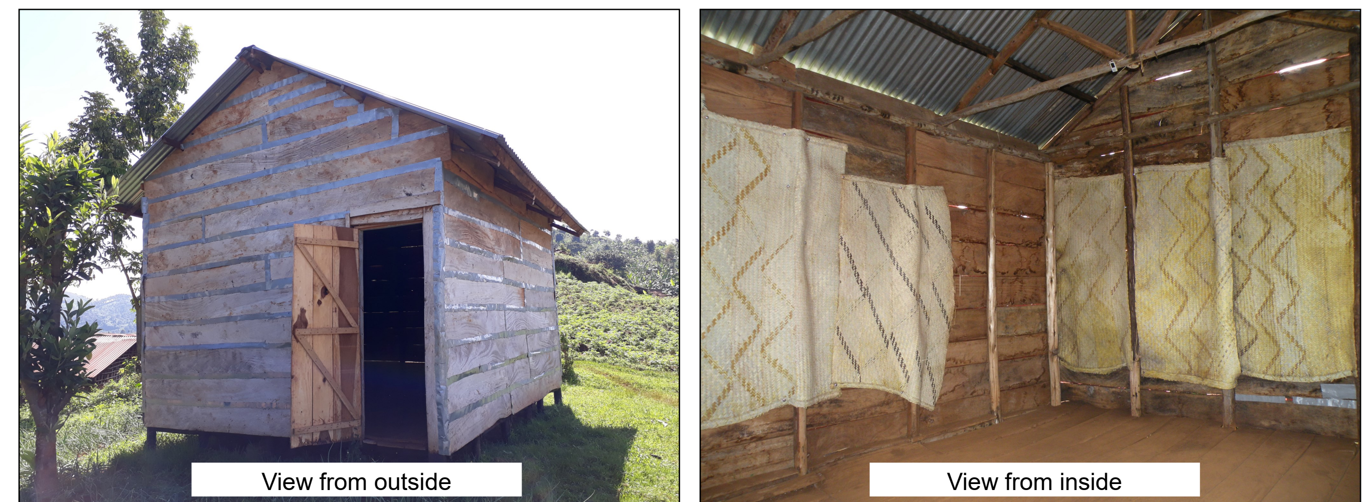
Figure 3: Improved individual ambient ware potato stores piloted in Uganda (8 t storage capacity, 10 years lifespan, unit cost of approximately USD 1,100).
