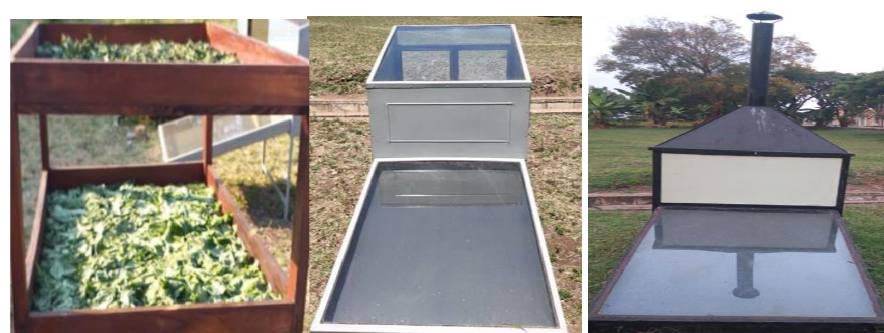
Fig. 1. Open sun, Indirect solar and Mixed solar driers
