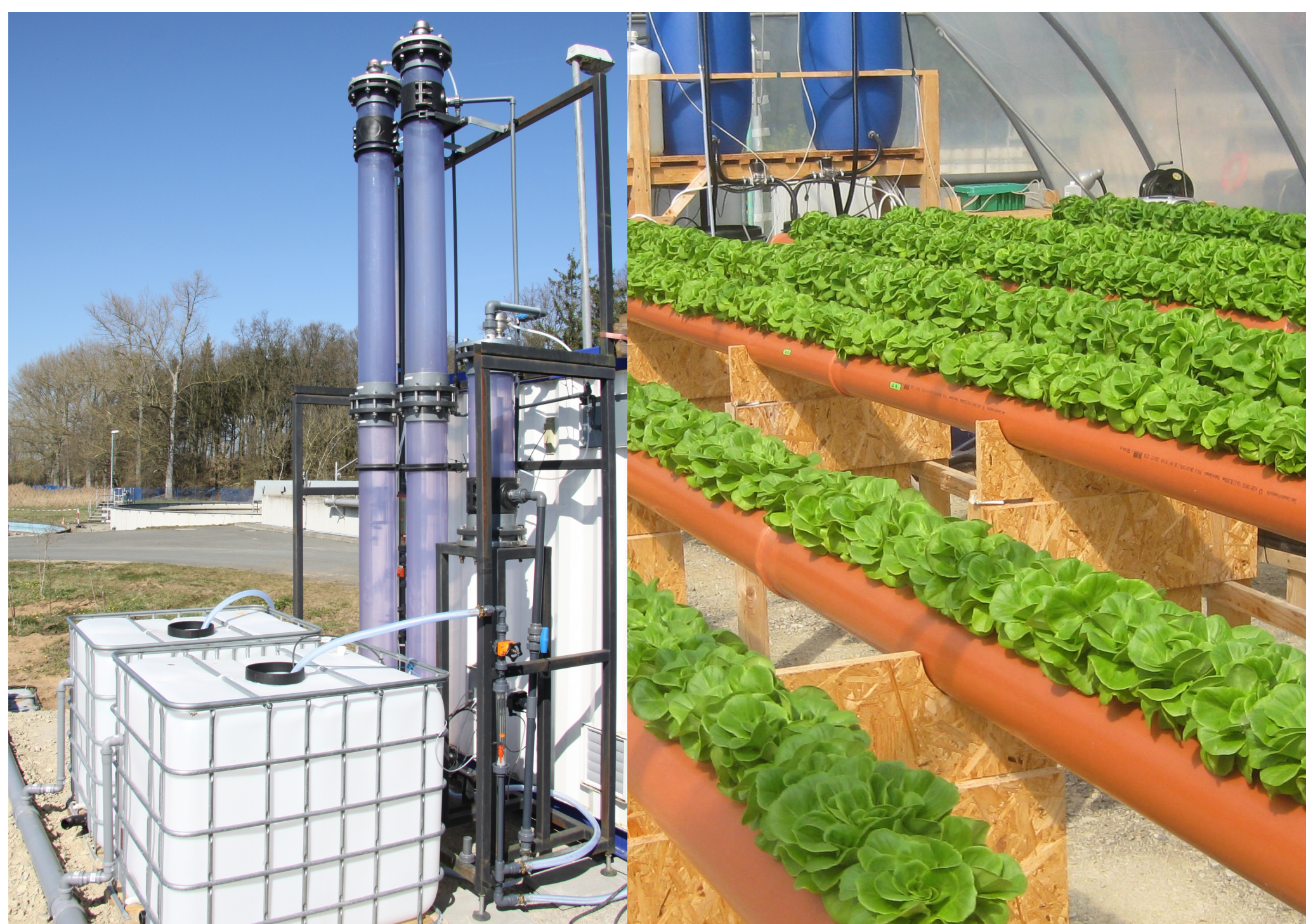
Experimental ozonation unit & lettuce grown with treated wastewater
