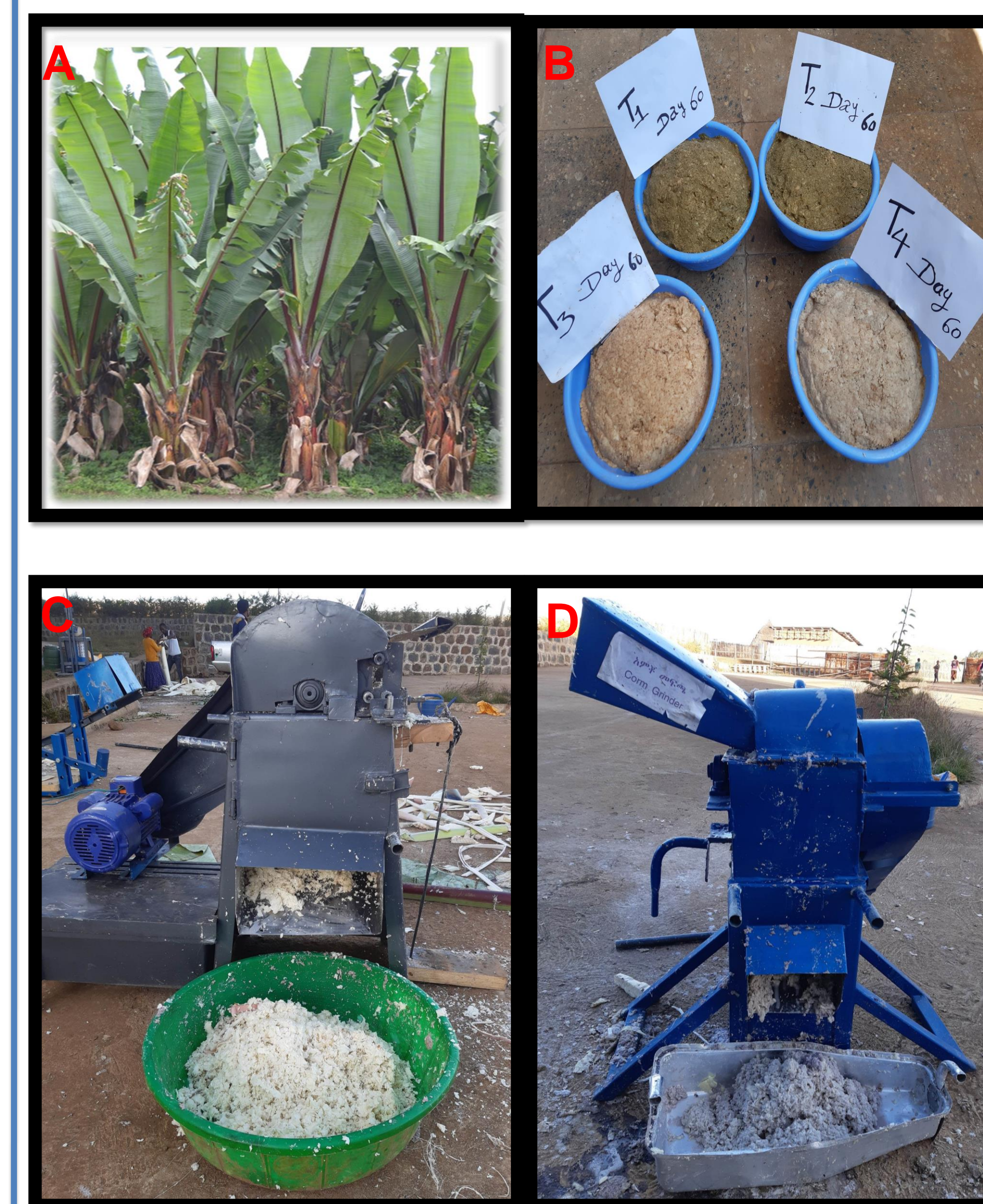
Fig. 1. Enset plant (A), fermented and fortified enset samples (B), enset pseudostem scraping machine (C), Enset Corm milling machine (D)
