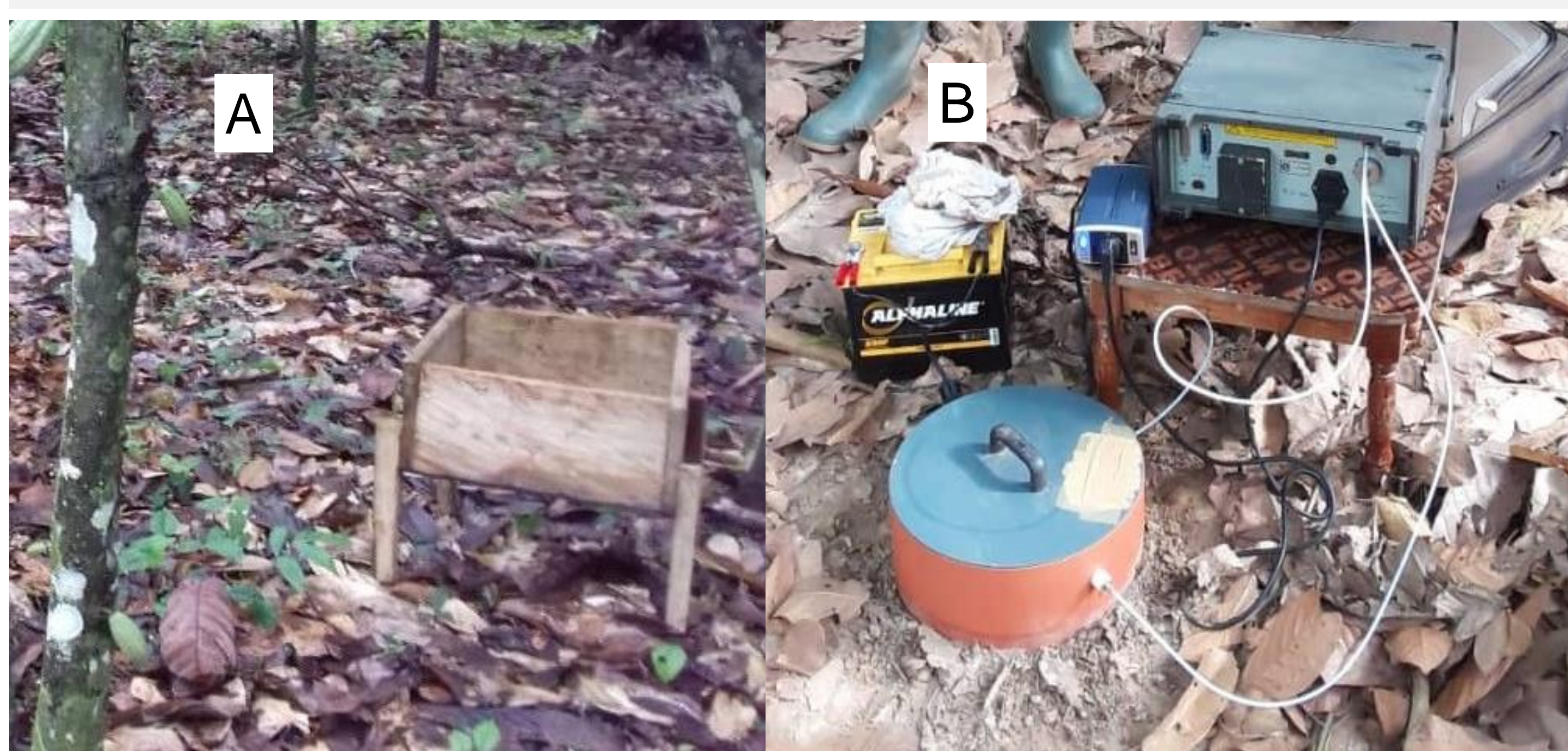
Figure 3 Wooden litterfall box (A) and photo-acoustic infra red gas analyzer (INNOVA 1312-5) (B)
