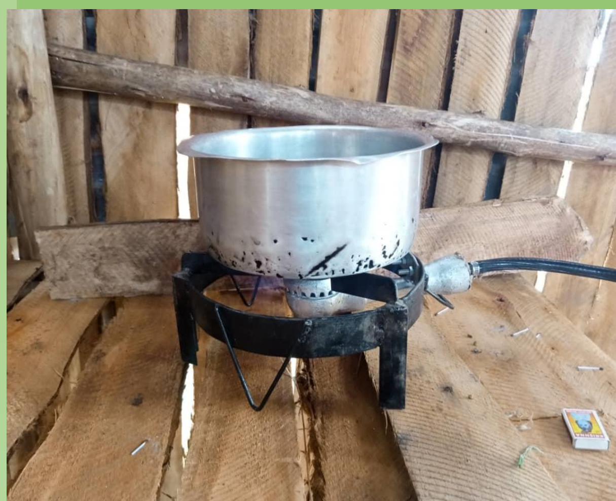
Figure 9: Boiling water using biogas from anerobic co-digestion of jackfruit waste with cow dung
