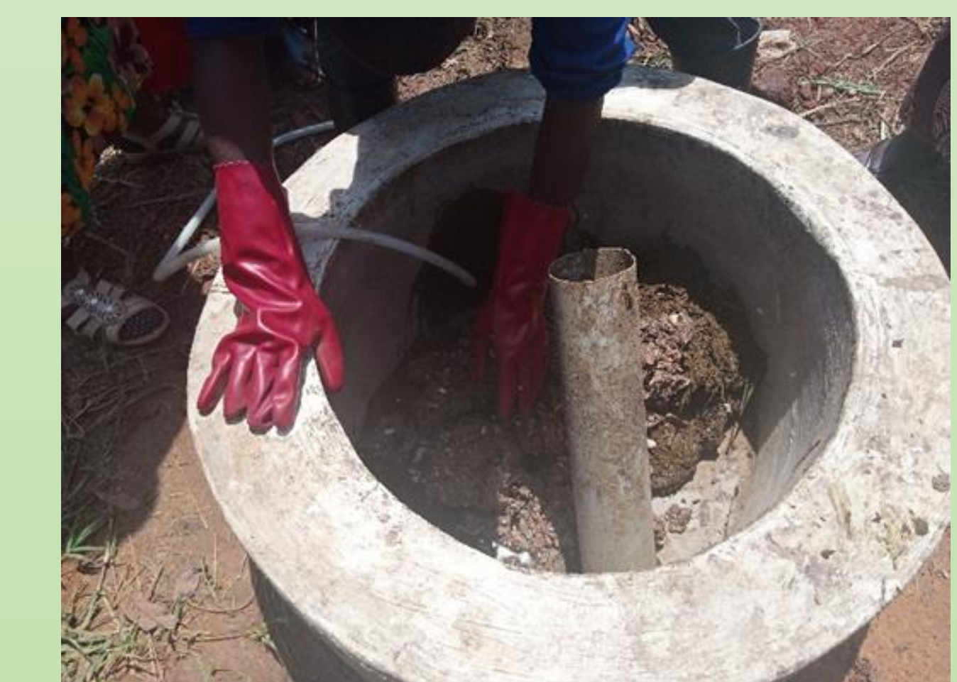
Figure 3: Mixing cow dung with water before anaerobic digestion
