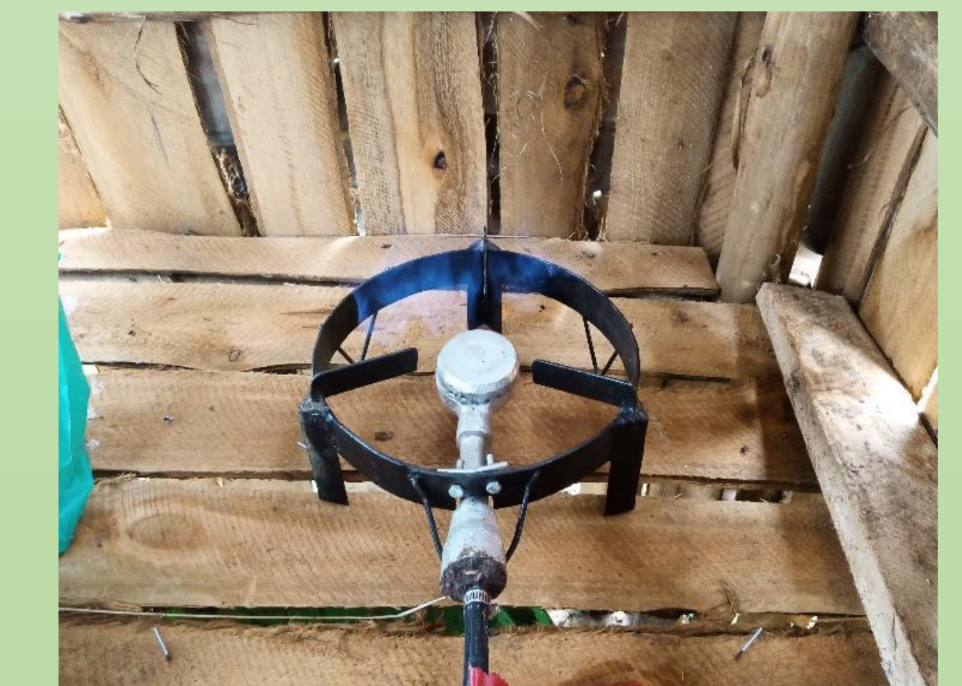
Figure 4: Biogas from the jackfruit waste and cow dung ready for cooking
