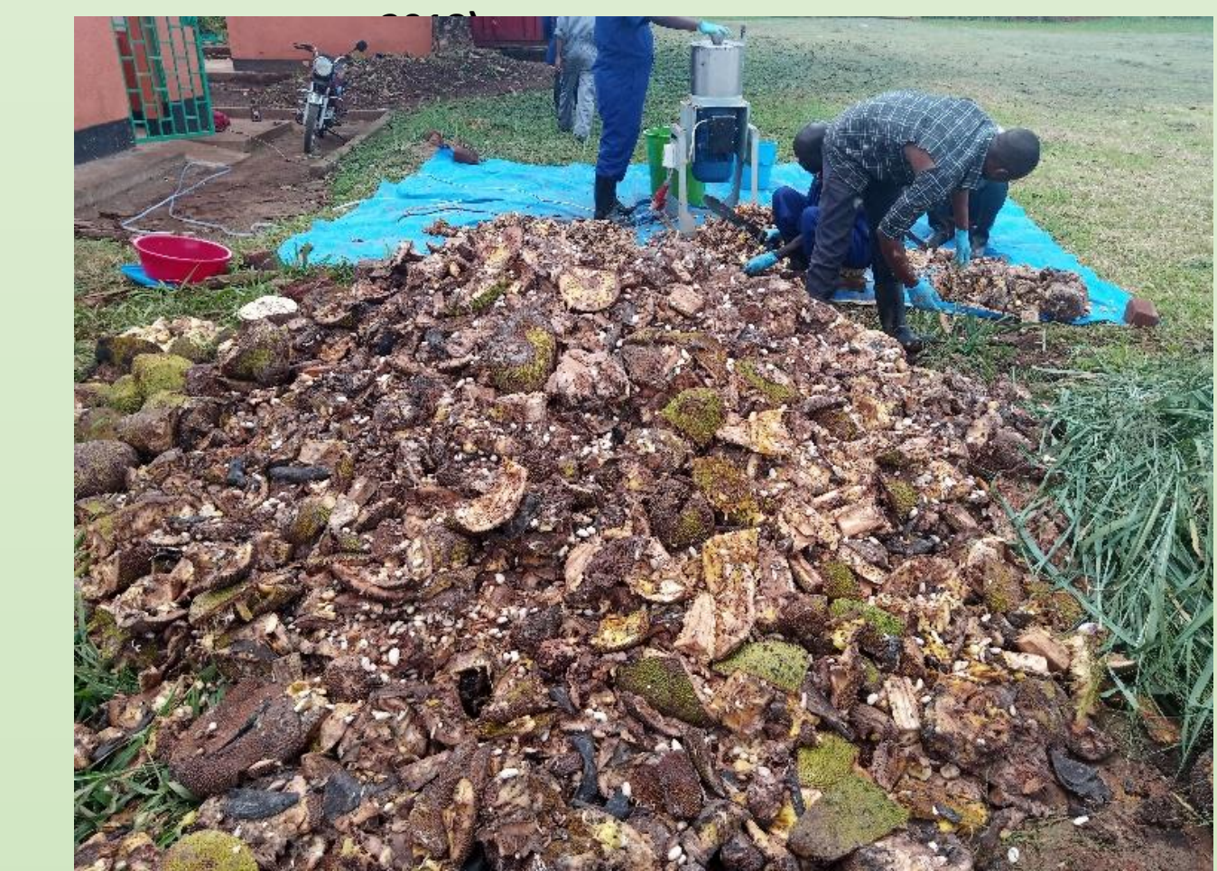
Figure 2: Reducing the jackfruit waste size before anaerobic digestion
