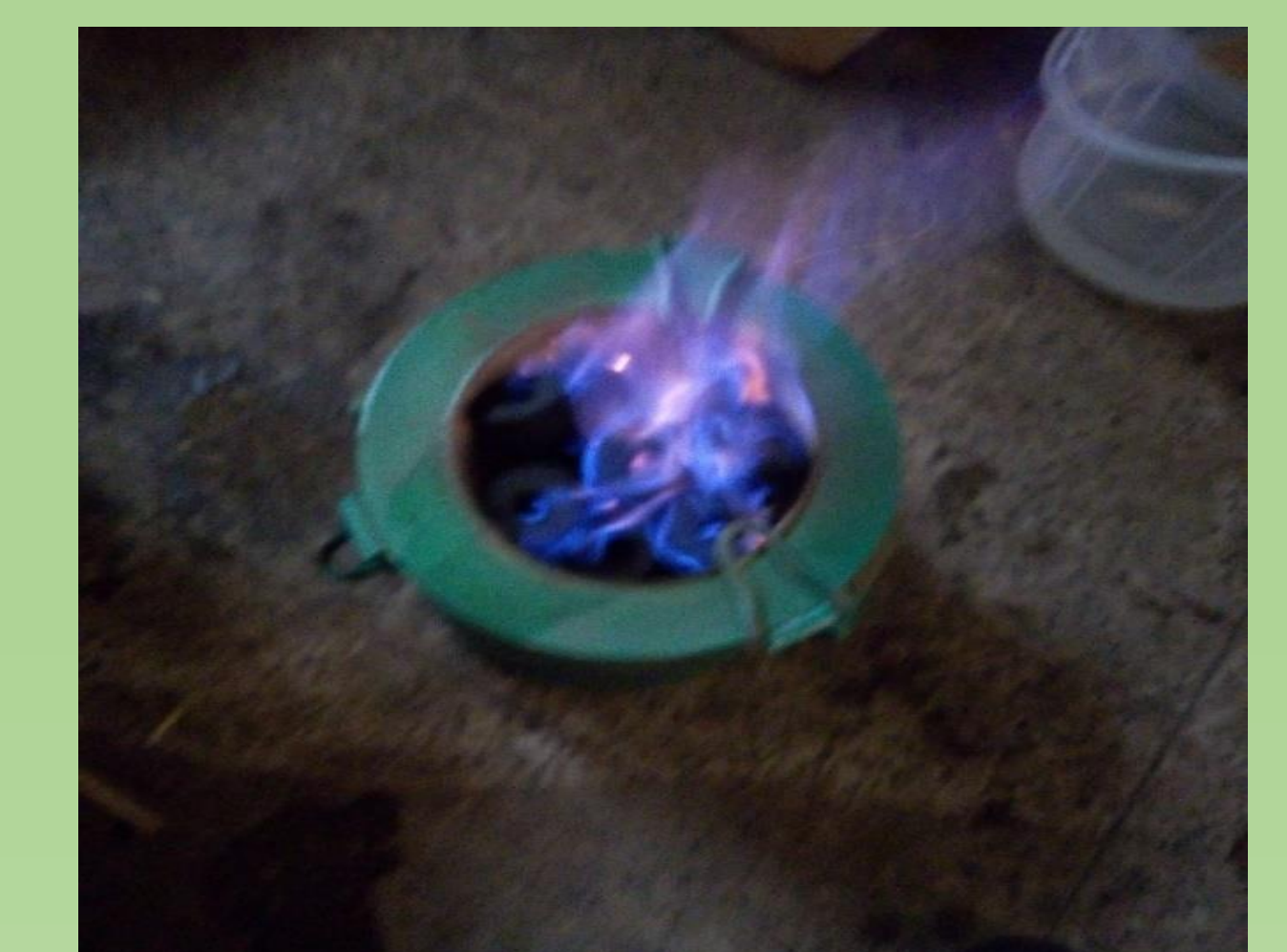
Figure 6: Jackfruit waste-based briquettes ready for cooking
