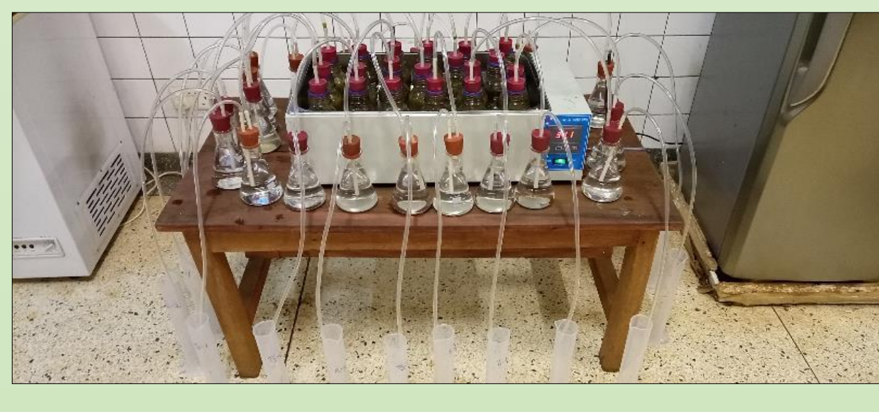
Figure 7: Lab-scale anaerobic digestion experimental set-up for biogas production
