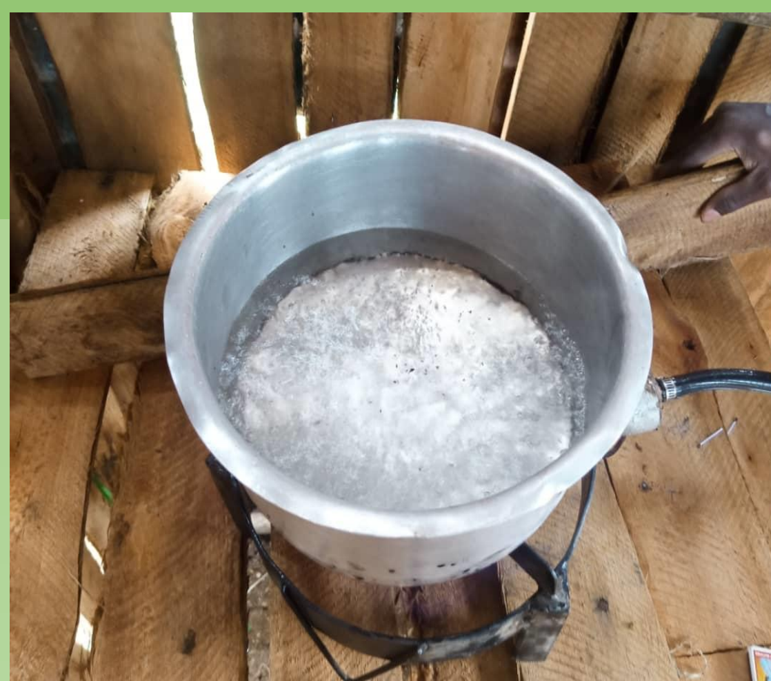
Figure 9: Boiling water using biogas from anerobic co-digestion of jackfruit waste with cow dung
