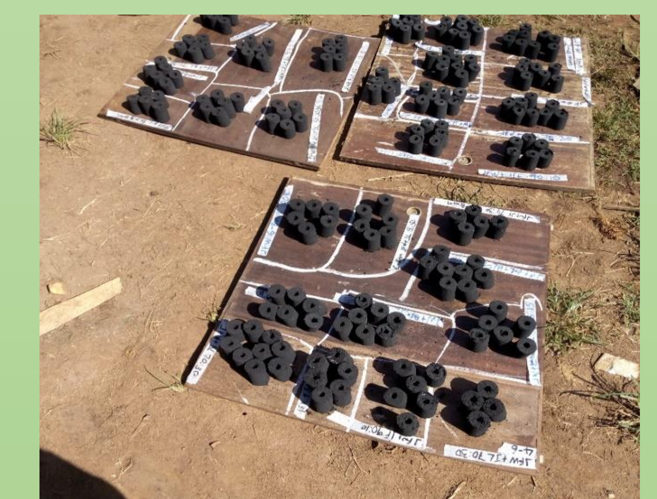
Figure 5: Sun Drying Jackfruit waste-based briquettes
