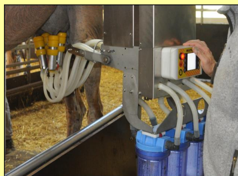
Fig. 4: StimuLactor (ST-C) for Camels during milking
