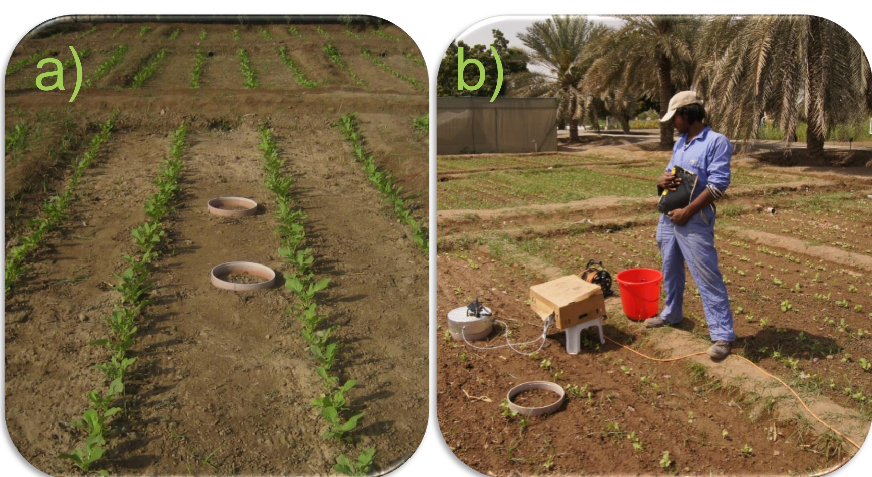
Figure 2 (a) Radish field with PVC ring installed for gas measurements and (b) gas measurement in the field
