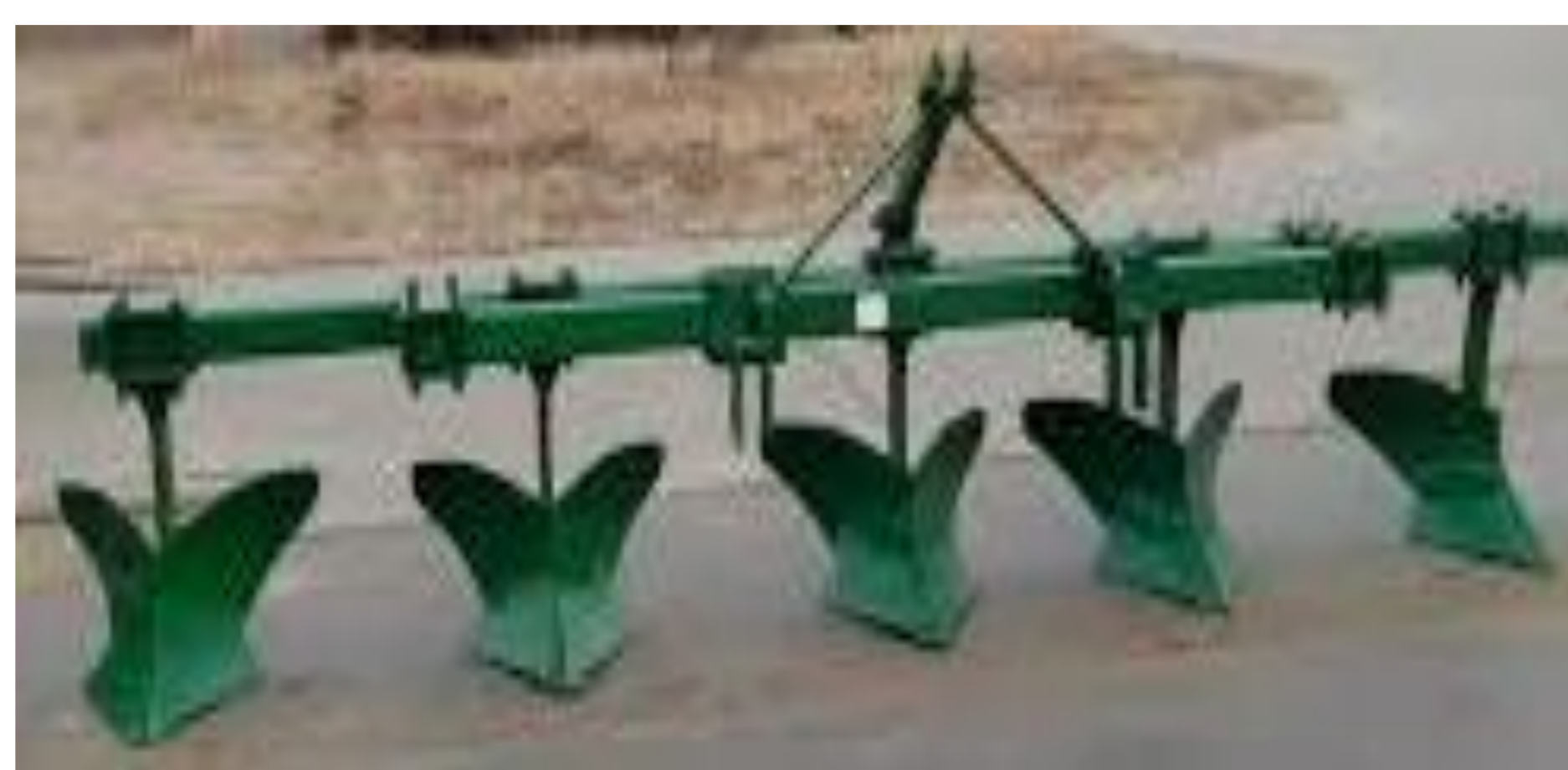
Fig.6 : Ridger plough for smoothing and leveling
