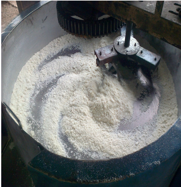
Fig. 1: Roasting of ‘gari’ in a ‘garifier’
