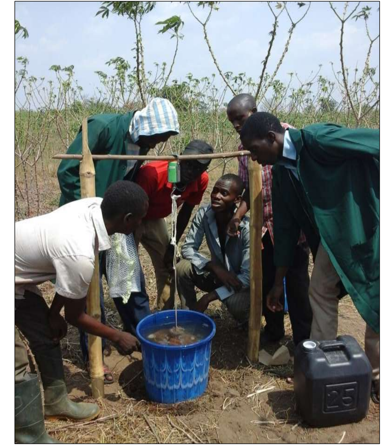
Determining cassava root starch content by the gravimetric method
