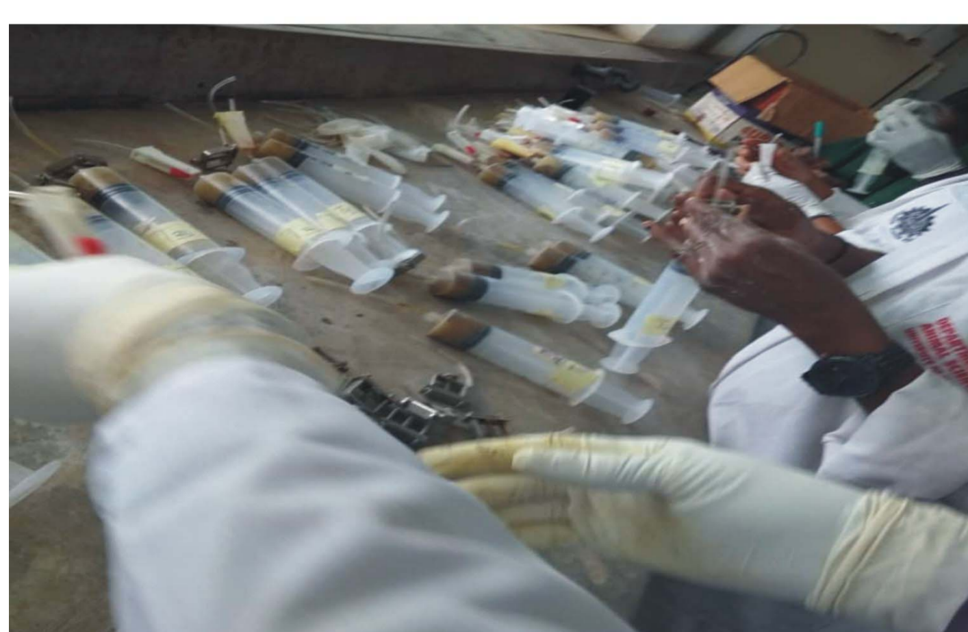
Pix 3: filling the syringe with inoculums and samples
