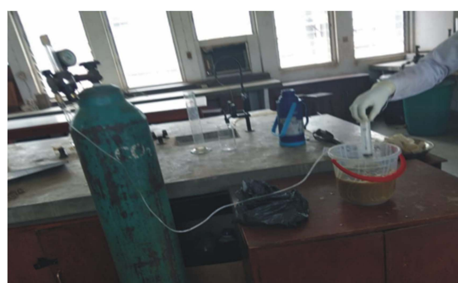
Pix 2: Flushing of the rumen liquor with carbon dioxide to make prevent the micro organisms from dying.
