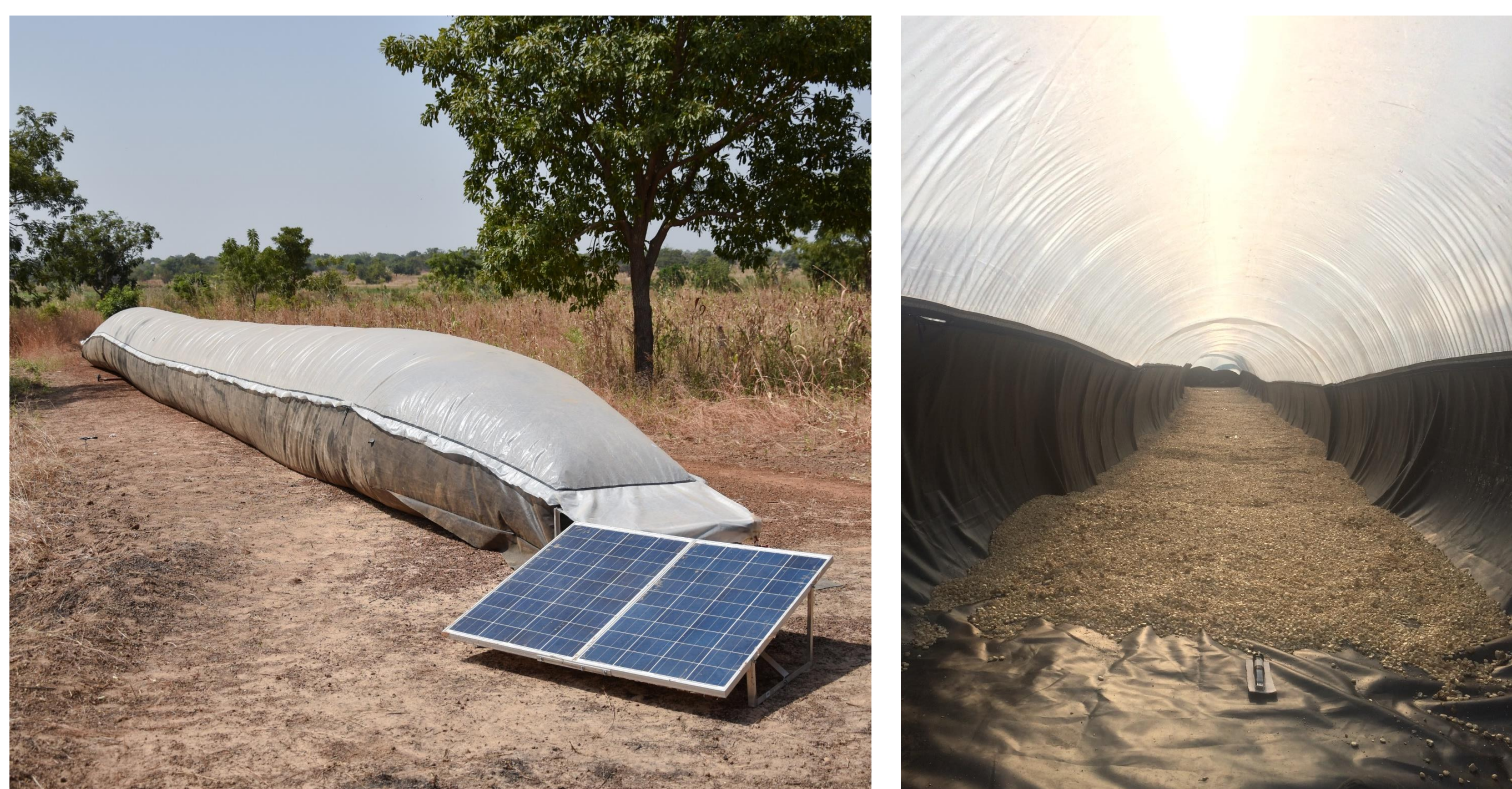
Fig 1. Inflatable Solar Dryer with nominal capacity of 1000 kg maize.
