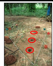
Picture 3: Holes of auger method inside the Voronoi triangle after root sampling (M3)
