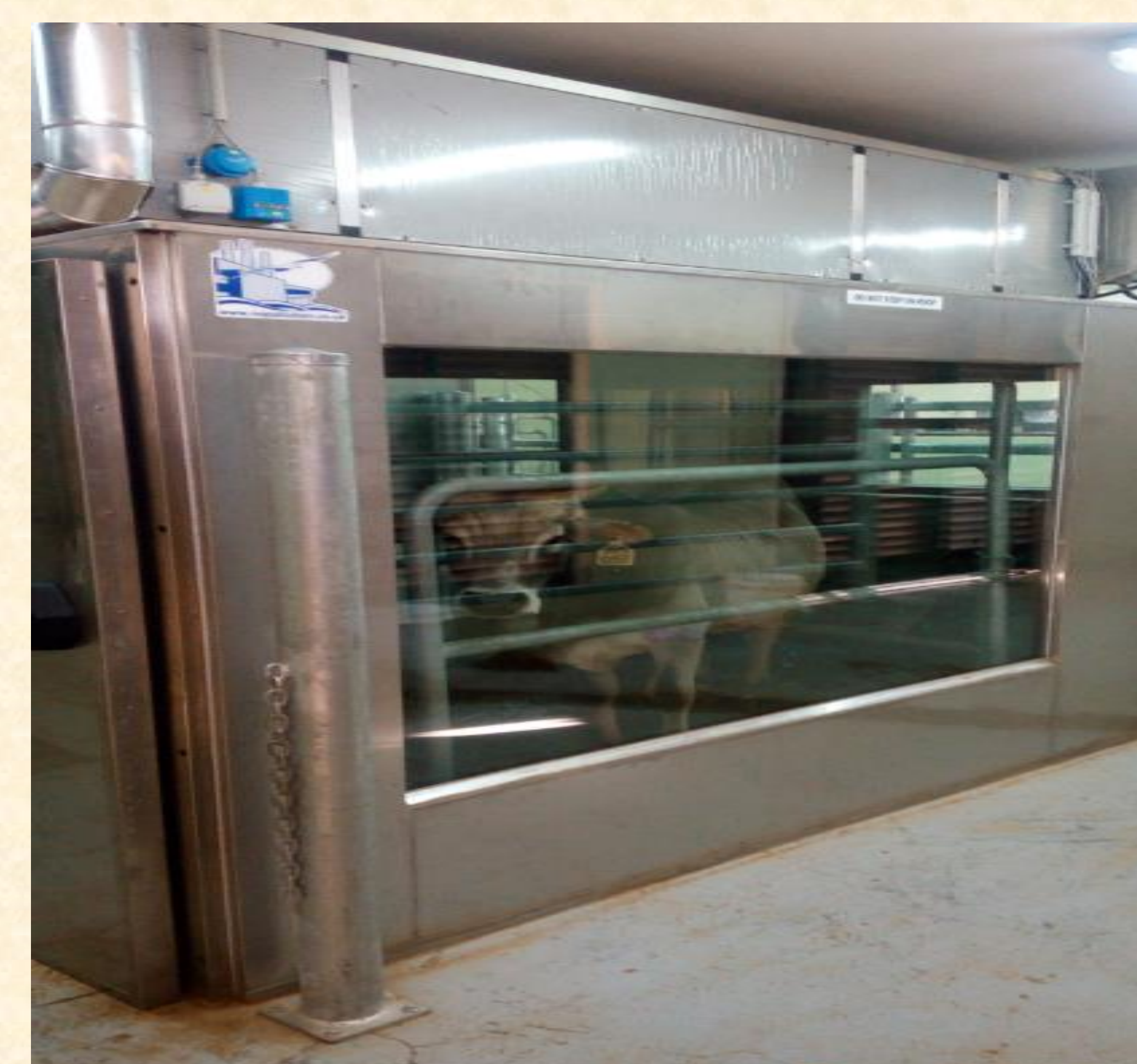
Figure 2 : Animal in the respiratory chamber during methane production measurements.
