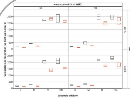
Fig. 1: Cumulated respiration ( $\mu\text{g CO}_2\text{-C g}^{-1}\text{ soil}$ ) of the two incubated soils (A & B) after addition of organic amendments at two different moisture and salinity levels ( $n=4$ ).
