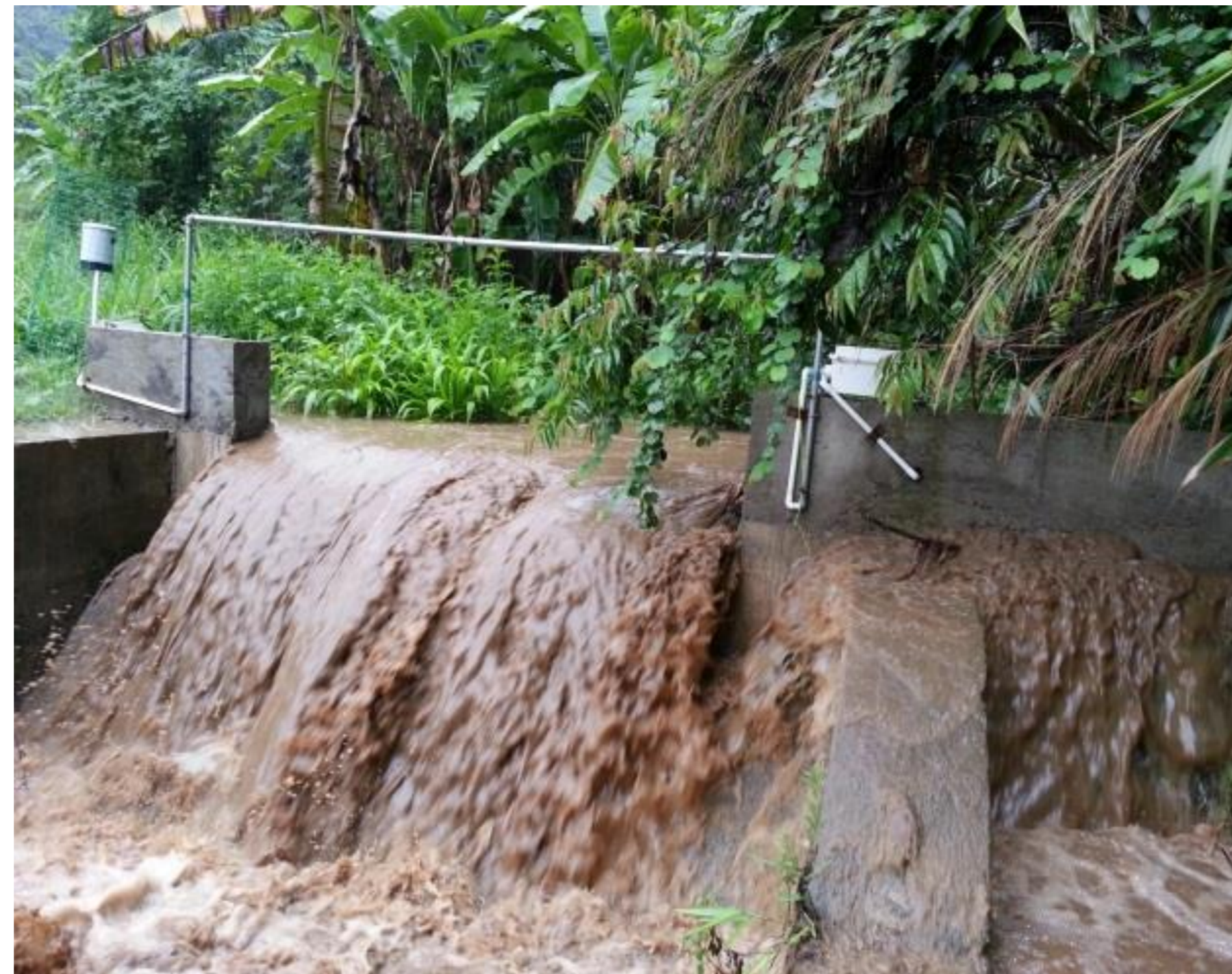
Figure 1: Hydrological station continuously measuring water level and turbidity at watershed outlet.
