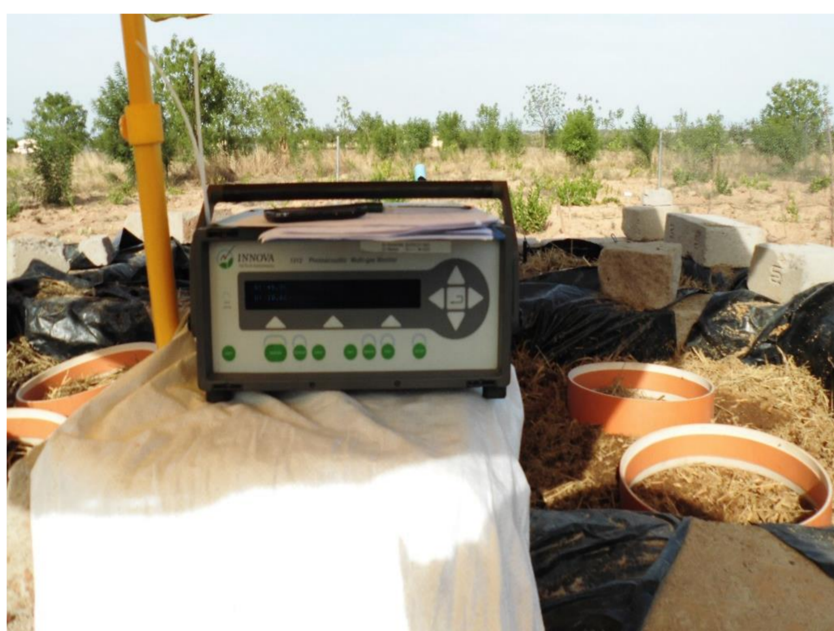
Figure 2 Photo-acoustic infrared gas analyser (INNOVA 1312-5)
