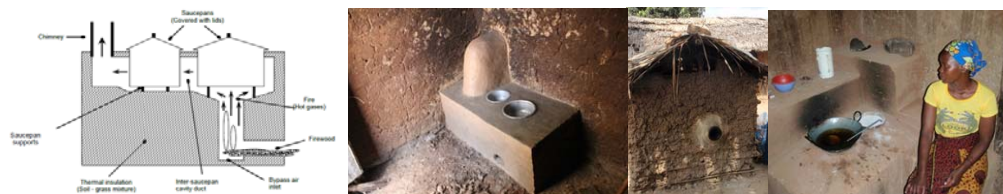
Figure 1: Stove scheme and pictures of ICS implemented, chimney and new ICS design
