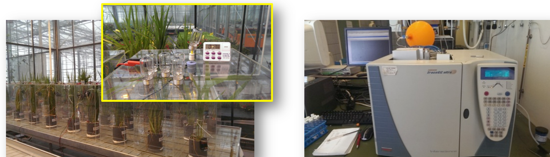
Fig. 3. Gas sampling and Gas Chromatography analyses
