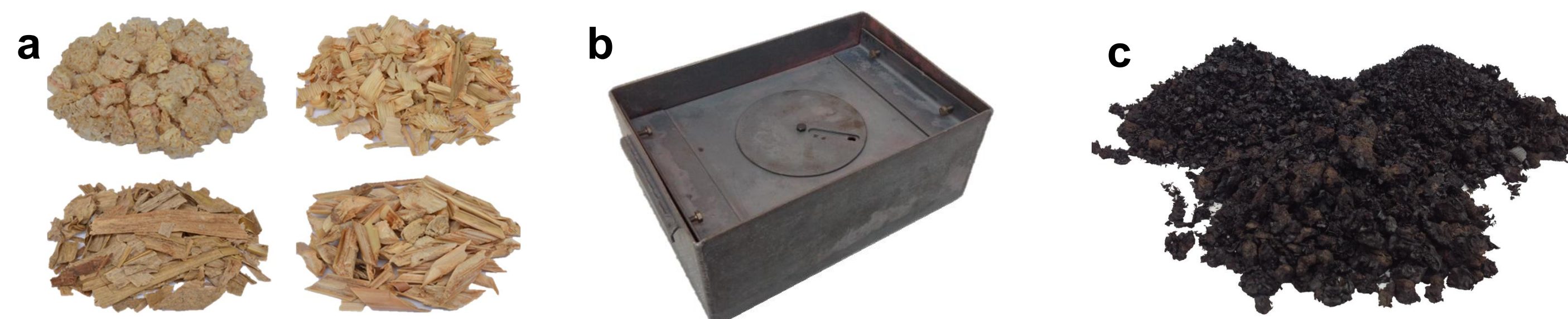
Fig. 1. (a) biomass fractions, (b) pyrolysis reactor, (c) cob biochar.
