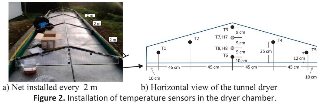
**Figure 2.** Installation of temperature sensors in the dryer chamber.
