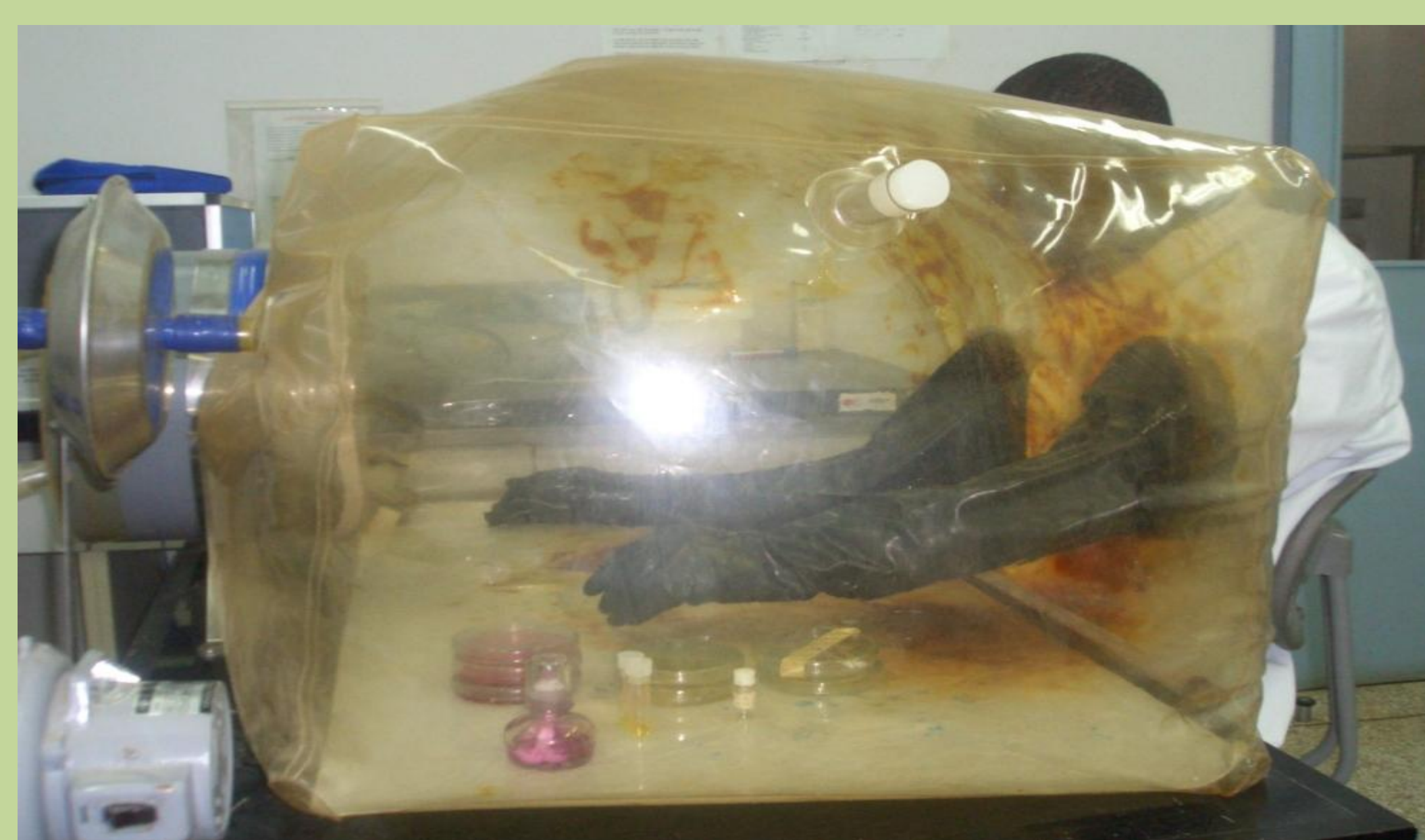
Figure 1: Improved anaerobic glove box using a vinyl isolator
