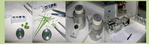
Osmotic potential measurement using a Wescor HR 33T (Wescor Inc., Logan, UT) automatic scanning dew point microvoltmeter with three sample chambers (Wescor C-52).
