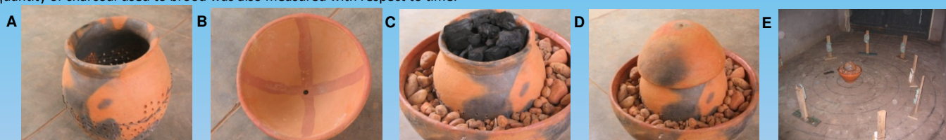
Plate 1: A- a perforated pot with gauze, B-a lid to the perforated pot, C- clay basin filled with pebbles and clay pot filled with 500g of charcoal , D and E-a fully set-up of the “Awudu” heater,
