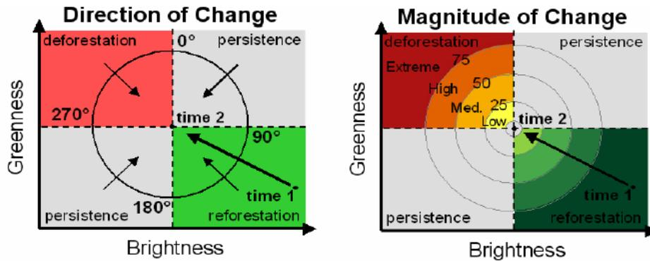
**Figure 2:** The process for detecting the direction of change (a) and the magnitude of change (b) within change vector analysis.
