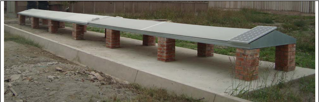
Figure 2: Solar tunnel dryer “Hohenheim type” installed at INIA Donoso, Hural
