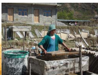
Figure 4: A woman making Nepali handmade paper out of Lokta bark in Everest Gateway Handmade paper Enterprise
