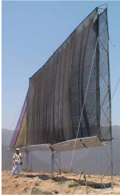
Fig. 1: "Eiffel" collector. 4x8x0.3m metal frame, two separated layers of metal frame, 2,256m of 1.5mm Raschel 50% net with 10 additional rubber string vertically installed in between
