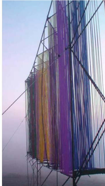
Fig. 1: "Eiffel" collector. 4x8x0.3m metal frame, two separated layers of metal frame, 2,256m of 1.5mm Raschel 50% net with 10 additional rubber string vertically installed in between
