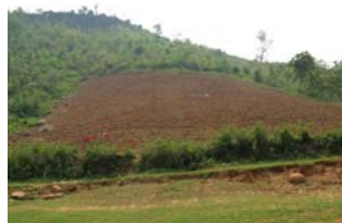
View of Field 1 before planting maize with Gerlach troughs and erosion pins installed to measure erosion and soil loss.
